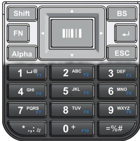
The function keys can be programmed to start an application. To program function keys tap
